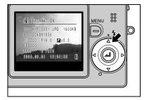
3 Press the shutter release button half way to return the camera to the original shooting mode.
